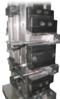
5-side machining: Multi-clamping (unfinished parts) in RKD 125 with hold-down pronged inserts
