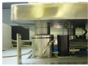
In order to guarantee reproducible measurements it was necessary to install air springs. The scale requires fast-acting and precise level control that also compensates the electrical effects of the glass hood.
