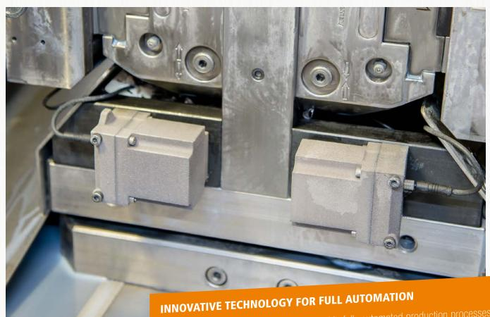
Wireless sensoring systems from AMF enable fully automated production processes for both clamping technology and modern handling and storage systems.
