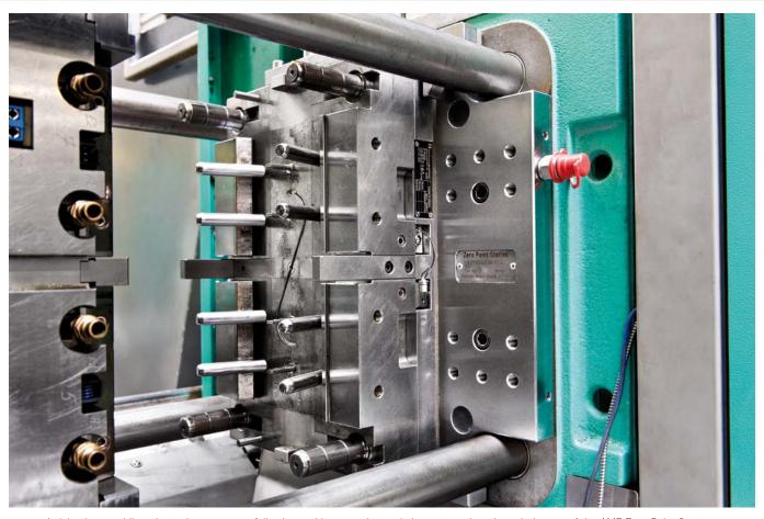
In injection moulding, the tools are successfully changed in a way that optimizes set-up time through the use of the AMF Zero-Point System.
