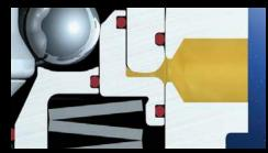
Process reliability - Clamping module always opens. A piston blockade is thus impossible (only Gonzales modules).
