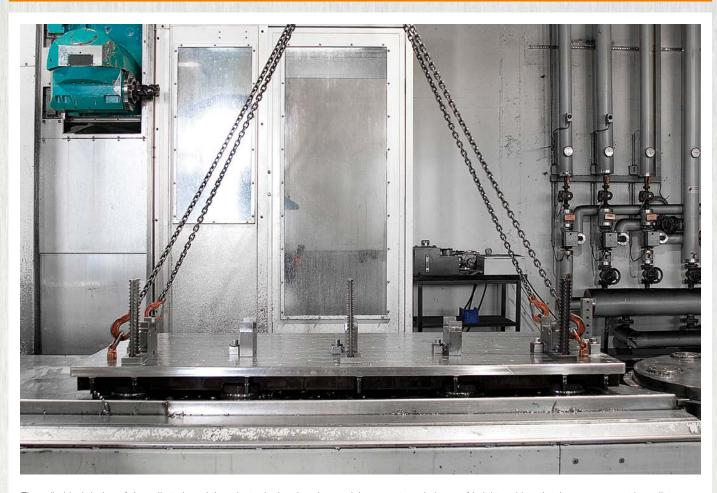
The cylindrical design of the pull-studs and the adapter in the clamping module guarantee a balance of height and length tolerances even at long distances.
