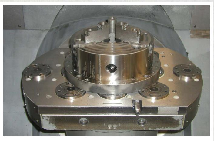
Simple changing of a 3-jaw chuck by means of the AMF zero-point system.
