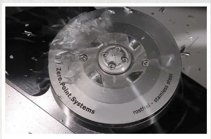
The integrated cleaning turbine blows off shavings and dirt reliably from contact surfaces.
