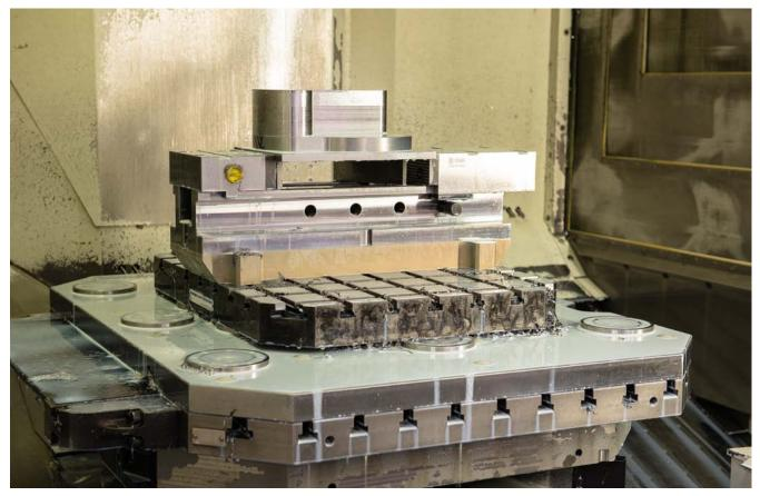
Thanks to the low installation height of our clamping modules, the assembly of the clamping device can be adapted flexibly to the respective machining height and workpiece.
