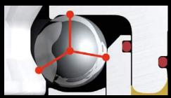
Power transmission by means of the threepoint principle! This optimised force distribution prevents shearing load on the balls.
