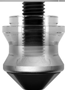
> The pull-stud in our zero-point system is the interface between the machine table and the workpiece or fixture. It ensures exact positioning and secure clamping. The resulting work forces are transferred through the pullstud to the clamping module.
