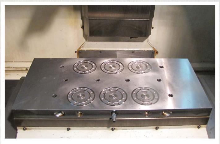
The cylindrical mating receptacle makes recessed installation of the clamping modules easily possible without any loss of precision.
