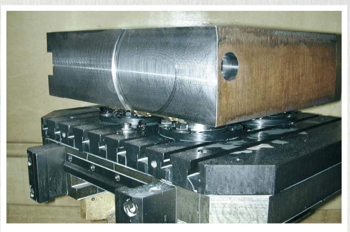
Surface-mounted clamping modules with clamping flanges for easy and flexible positioning of the T-slot tables.
