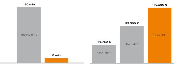
Tooling times drastically reduced from 120 mins to 8 mins - through the use of the AMF Zero Point System.
