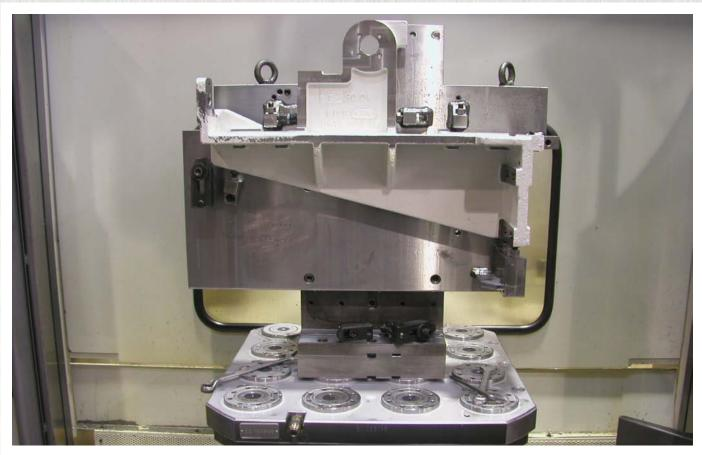
The AMF zero-point system offers a secure fit during drilling operations under unfavourable lever ratios.
