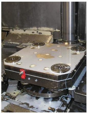
The module interior is completely sealed. As a result, the system is optimally protected against liquids and dirt.
