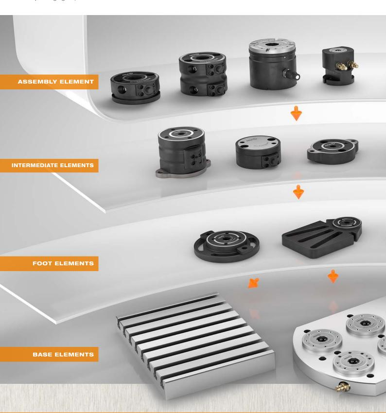
The modular height adapters consist of three levels. The foot elements form the interface to the existing machine table. Building on this and with the use of intermediate elements, every clamping height can be achieved and, by combining different sizes, adapted flexibly to the contour of the workpiece.
