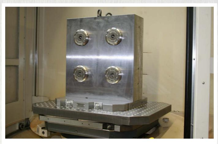
Integration clamping module as flange version for installation on clamping profiles.
