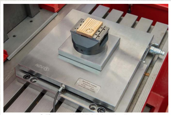
The AMF zero-point system is the standard interface here between various machines.
