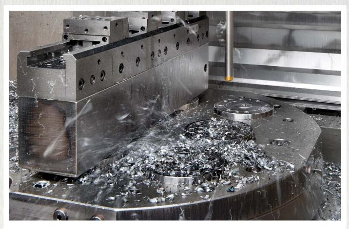
AMF-Clean-Stick in use: automated cleaning of clamping fixture and machine table.
