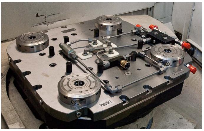
Combined application between zero-point clamping technology and hydraulic media transfer.
