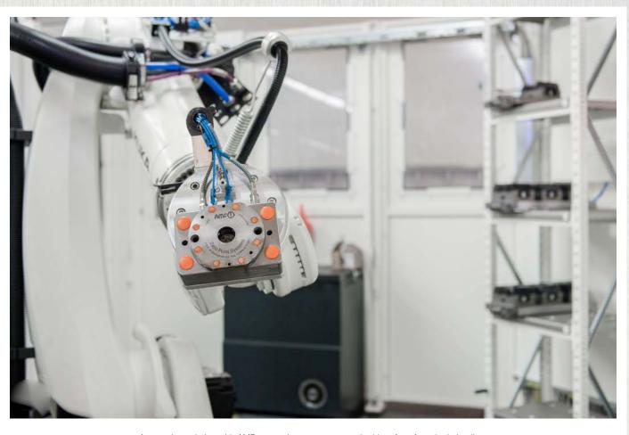
Automation solution with AMF zero-point system as standard interface for robotic loading.
