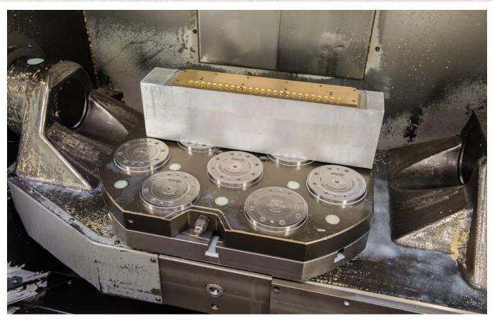
Whether at a standard module distance of 200 x 200 mm or in any other pitch spacings and arrangements of the clamping modules, the AMF zero-point system can be adapted to any practical requirement.
