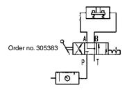
Circuit: hydraulic clamping module with blow-out
