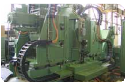
Milling machine for the production of tensile tests
