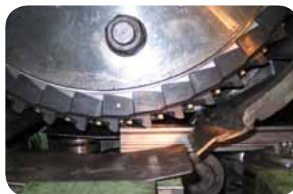
Milling machine for the production of linear guides
