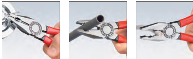
Grip zone for flat workpieces Grip zone for round workpieces Cutting edges for wires and cables
