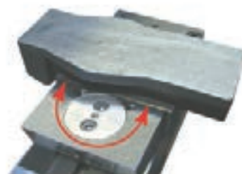
Jaws with 4 compensating supports corrugated; Compensation \pm 9^\circ , movable jaws floating, without hold-down for clamping of forgings
