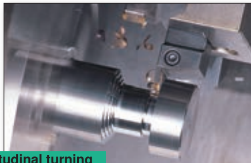
Longitudinal turning and Recessing
